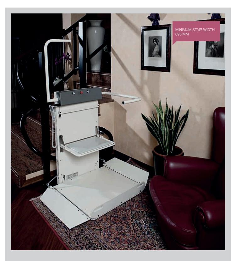
Minimum stair width895 mmPlatform dimensionsmin 750xPlatform dimensions225 kg (dMaximum load capacity225 kg (dMax. gradient0° - 60°Min. overall dimensions with platform closed305 mmMinimum rail overall dimensions95 mmElectrical consumption1,1/1,5 kInstallationindoor/ouSoft-start and soft-stop systemstandardSlow down at bendsstandard
