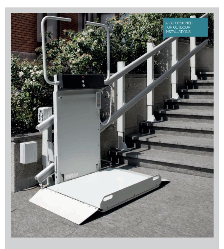
Minimum stair width Platform dimensions Maximum load capacity Max. gradient Min. overall dimensions with platform closed Minimum rail overall dimensions Control circuits voltage Speed Soft-start and soft-stop system 850 mm min 750x600 / max 1250x800 250 kg (daN) 10° - 45° 350 mm 115 mm 24 V DC 0,1 m/s max standard
